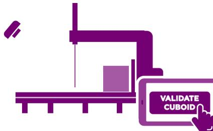
Load any nested cuboid on the table. The system is ready for cuboid identification, using the integrated\* SmartCut camera. Press the "Validate Cuboid" button in the Smartcut device to initiate the process.
